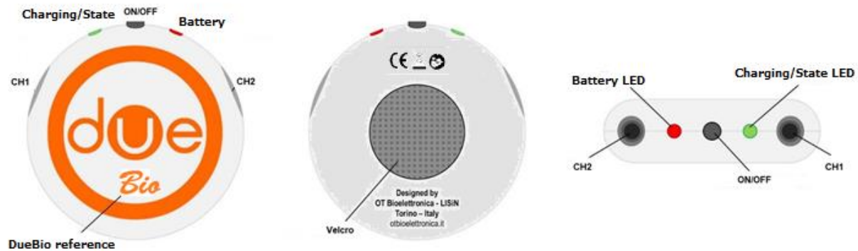
FIG. 7.4: Front, back and side view of DueBio probe.
