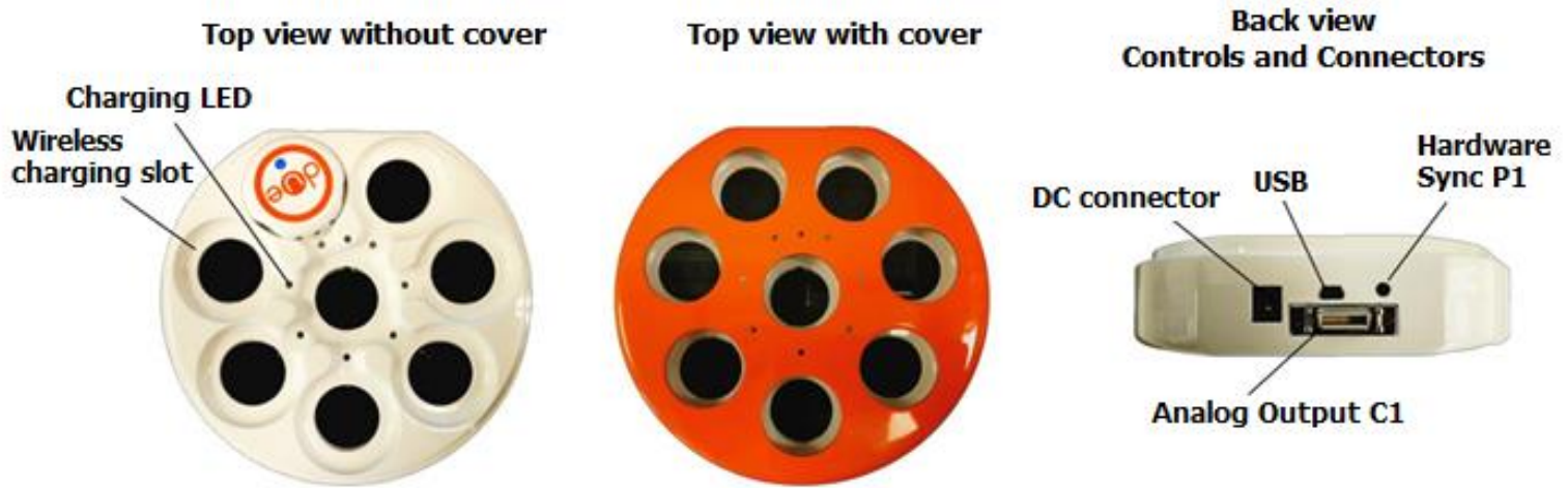
FIG. 7.6: Top and Back view of DueStation.
