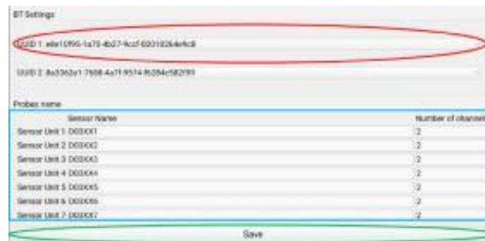
FIG. 8.7: Form for the connection options, UUID list (red circle) indicates the UUID used to connect the probes, name of the probes (blue circle), save button (green circle).
