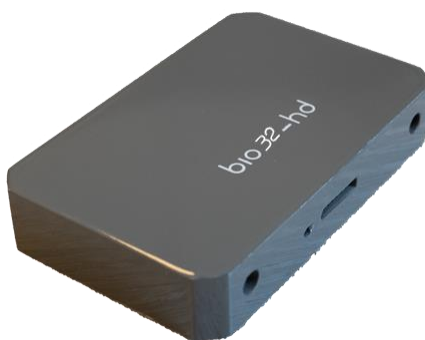
FIG. 8.6: Bio32-HD probe for electrode grids with 32 channels
