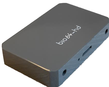
FIG. 8.5: Bio64-HD probe for electrode grids with 64 channels
