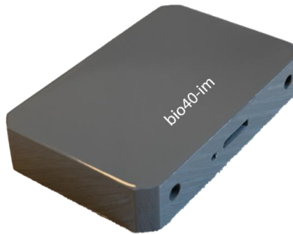
FIG. 8.8: Bio40-IM probe for 40 intramuscular signals
