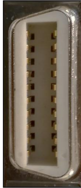
FIG. 8.9: Connector C1, Analog output and Trigger input (micro D Sub 20 poli – N. 3M-10220-6212PL).
