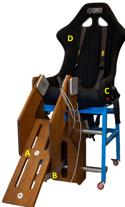
Fig. 1. The dinamometer COR1. A: adjustable plate where the leg is positioned and fixed. B: anchoring blade. C: seat sliding system. D: seat with belts.
