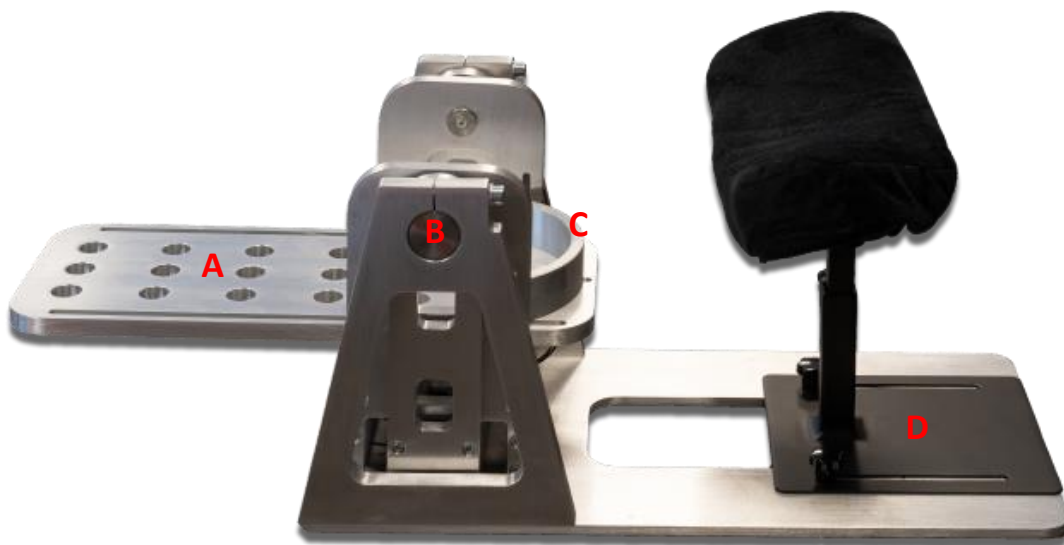
Fig. 1. The DinamometroGC and its parts: A = plate, B = pivot, C = heel/elbow support and D = positioning system for supporting the arm/leg.
