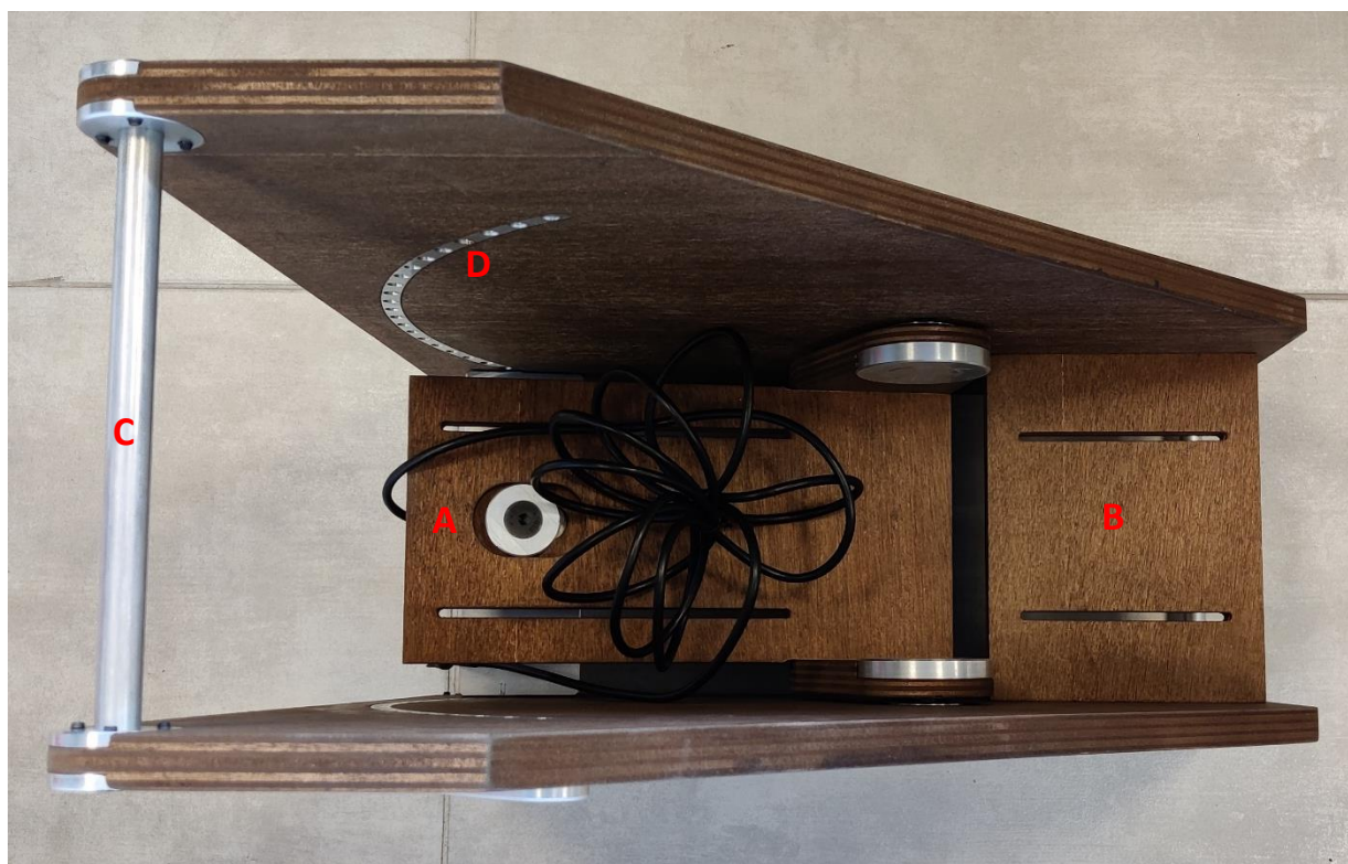
Fig. 1. The ergometer MUC1. A: the armrest. B, C and D: positioning system for the forearm.
