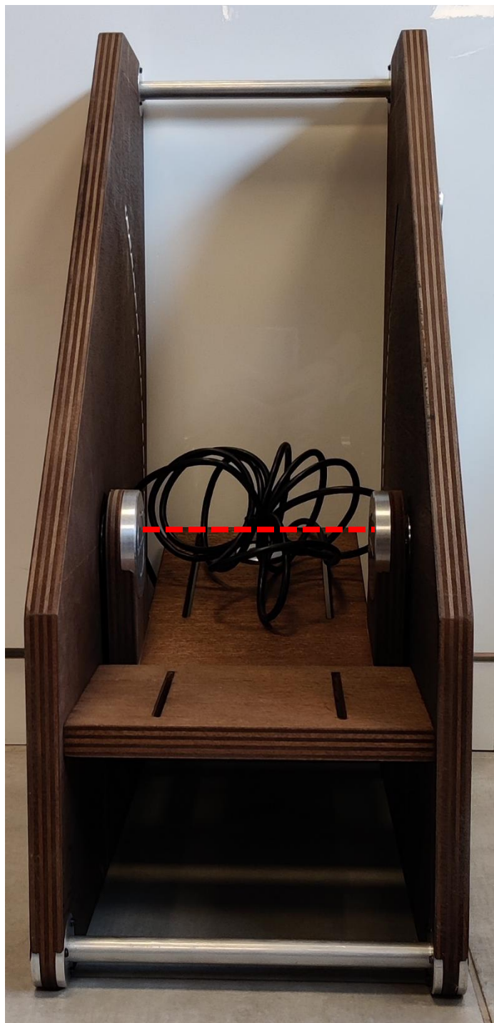
Fig. 2. Alignment between elbow and dinamometer centers of rotation.
