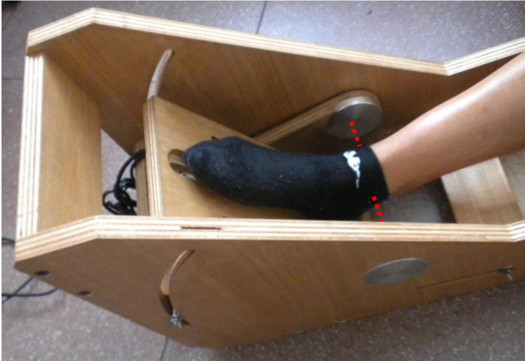
Fig. 2. Alignment between ankle and ergometer centers of rotation.
