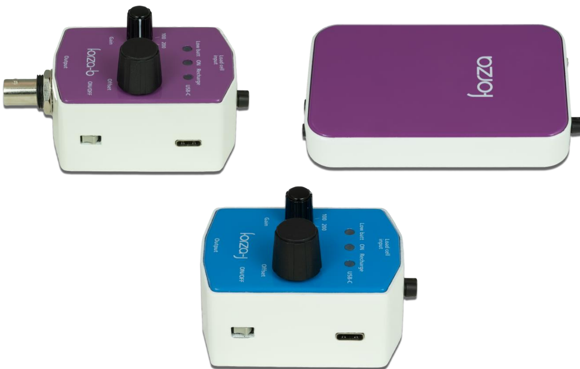
Fig. 6. Forzab, forza and forzaj load cell amplifier.
